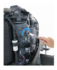
10. Carefully install the spark plugs by hand to avoid cross-threading. Tighten 1/8—1/4 turn after the spark plug seats.
