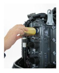
9. Pour a teaspoon of engine oil into all the spark plug holes to lubricate the inside of the cylinders.
