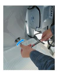
5. After draining the oil, install the drain bolt and new sealing washer, and tighten the bolt securely.
