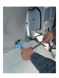
4. Place a suitable container under the oil drain bolt, remove the engine oil drain bolt and washer. Drain the engine oil until the flow of old oil reduces to a trickle.
