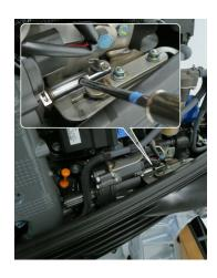
Insert the phillips screwdriver with the grip of the tool kit into the hole of the shift actuator.
