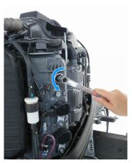
Remove all the ignition coil wire connectors, ignition coils and spark plugs.
